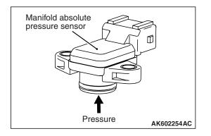
The manifold absolute pressure sensor is installed in the intake manifold. Manifold absolute pressure sensor uses a piezo resistive semiconductor to output the voltage according to manifold absolute pressure to ECM. ECM uses this output voltage to compensate fuel injection volume according to manifold absolute pressure. Sensor properties are as shown in the figure.
