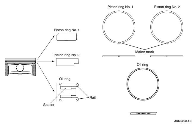
The piston rings consist of No. 1 and No. 2 rings and an oil ring.
