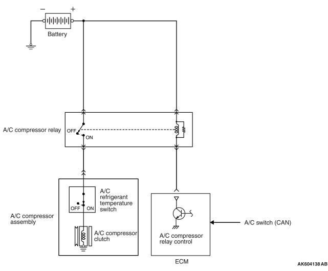
The ECM turns on the power transistor when the A/C switch ON signal is input by the A/C-ECU through the CAN. This allows the A/C compressor relay to be ON and to be operated. During the high load operation, such as the acceleration with the fully opened accelerator, the ECM secures the acceleration capability by turning off the A/C compressor relay for the specified period to produce no load on the A/C compressor.
