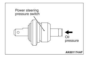
A power steering pressure switch is installed on the power steering oil pump. The power steering pressure switch uses a contact switch to detect the power steering oil pressure. When power steering oil pressure rises due to operation of the steering wheel, the power steering load switch outputs an ON signal to ECM. ECM performs idle-up according to the voltage and prevents reduction in engine speed due to power steering load and so maintains stable idle speed.
