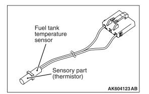
The fuel tank temperature sensor is installed to the fuel pump module. The fuel tank temperature sensor detects the temperature inside the fuel tank using the resistance change in the thermistor and outputs the voltage to the ECM in accordance with the temperature inside the fuel tank. The ECM monitors the evaporative leak in accordance with the fuel tank temperature. The sensor characteristics are as shown in the diagram.
