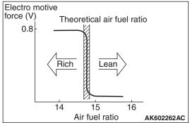
This sensor uses the oxygen concentration cell principle of solid electrolyte (zirconia) and displays the property of sudden change in output voltage near theoretical air-fuel ratio. This property is used to detect oxygen density in exhaust gas. Feedback to ECM allows it to judge whether air-fuel ratio is rich or lean compared to theoretical air-fuel ratio.
