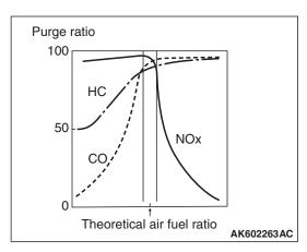
This allows ECM precise feedback control to get theoretical air-fuel ratio with best cleaning efficiency of 3-way catalytic converter.
