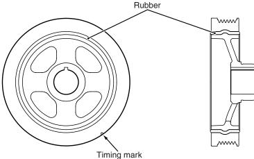
The pulley is made of cast iron.
