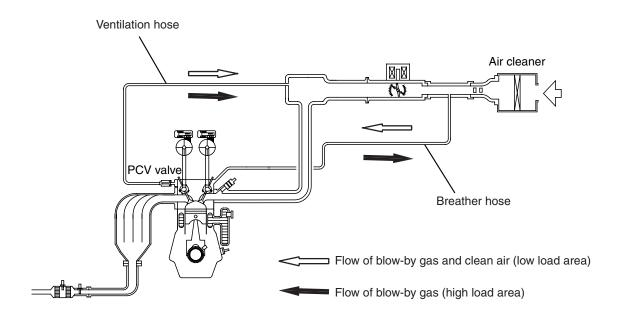
A blow-by gas reduction device prevents blow-by gas from being expelled into the atmosphere and is of closed type. A positive crankcase ventilation (PCV) valve is provided in the ventilation hose from the rocker cover to the intake manifold. During low load driving, clean air is supplied to the crankcase by the air intake hose via the breather hose and rocker cover, and it mixes with the blow-by gas in the crankAK604142AB
