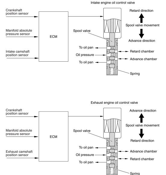
MIVEC allows the optimum valve timing to be controlled in accordance with the engine operation and the idling stability to be improved, as well as the output and the torque to be better in all the operation ranges.
