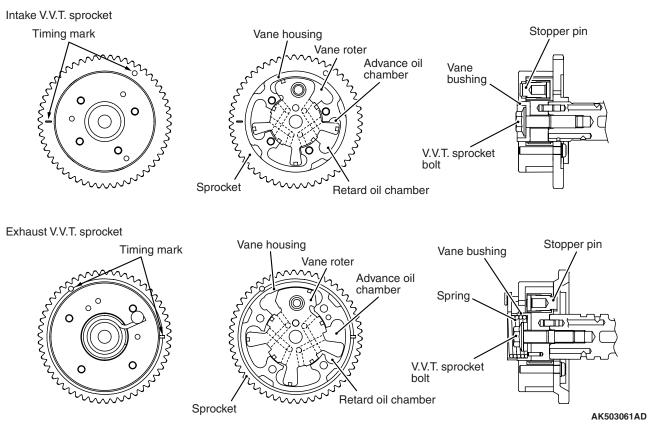
The engine oil control valve controls the hydraulic pressure in order to move the vane rotor in the V.V.T. sprocket to optimally control valve timing.
