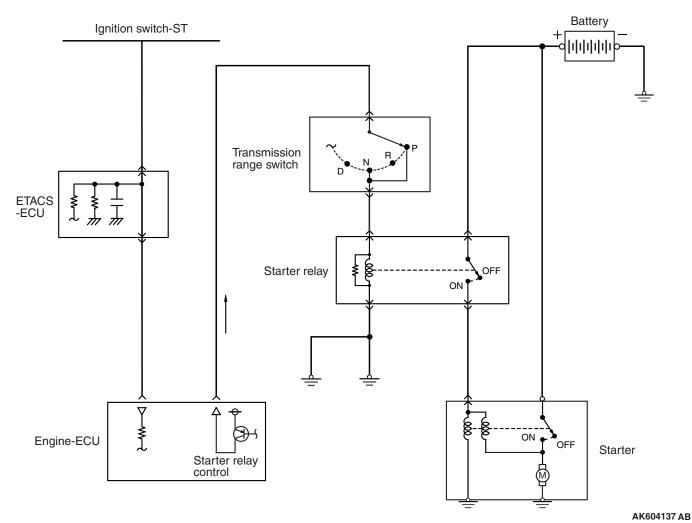
When the ignition switch-ST signal is input, ECM turns ON the power transistor for control of the starter relay.
