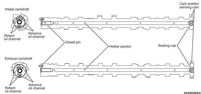
The camshaft are hollow for weight reduction. Each camshaft is provided with an oil passage to guide the hydraulic pressure from the engine oil control valve to the V.V.T. sprocket. A cam position sensing cam for detecting the cam position (used by the cam position sensor) is integrated at the back of each camshaft.
