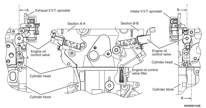
The MIVEC consists of the parts shown in the illustration. This system continuously varies and optimally controls the opening and closing timing of the individual intake and exhaust valves, in order to improve torque and power output in all speed ranges.
