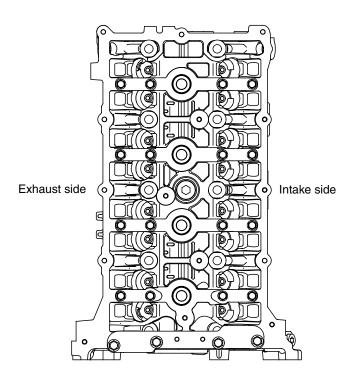
A cylinder head made of an aluminum alloy, which is lightweight and offers a high level of cooling efficiency, has been adopted. A pentroof combustion chamber with a center spark plug has been adopted. It has a small valve compound angle to realize a compact chamber.
