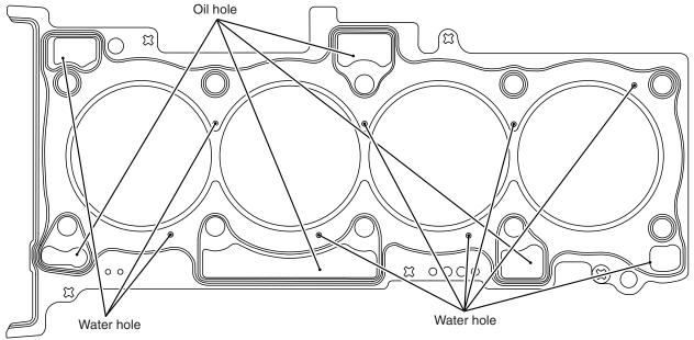
A dual-layer, metal type cylinder head gasket that excels in heat resistance and sealing performance has been adopted.
