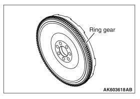
A cast iron ring gear is a shrink fit in the iron casting of the flywheel.
