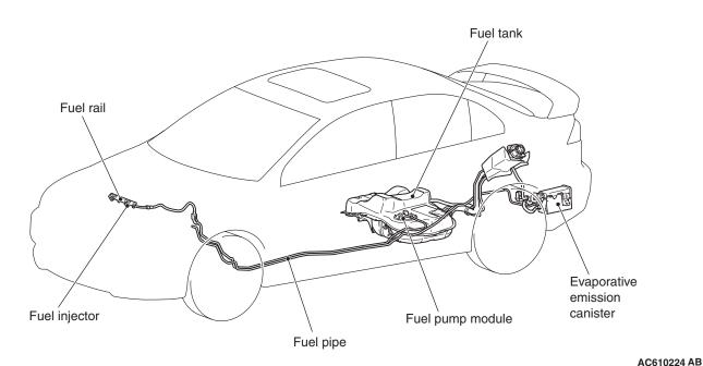
This fuel system is designed with consideration for global environment protection to ensure safety at a collision, reduce weight, and improve reliability and quality. This system has the following features:
