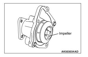
M2140003000168 The water pump is the centrifugal, impeller type that is installed in front of the cylinder block. It is driven by the drive belt.
